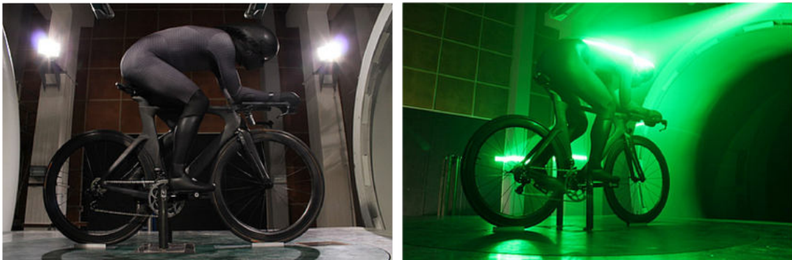
Figure 5.1: parts of Ridley Bikes' road bike and André Greipel's Lazersport helmet were measured and analyzed by the PIV system.
