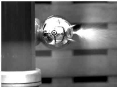
Corona discharge in air at the terminal of a transformer at 163 kV. With friendly permission of: Laboratory of High Voltage Engineering and Switchgear Technology, Technische Universität München, Munich, Germany [www.hsa.ei.tum.de](http://www.hsa.ei.tum.de)
