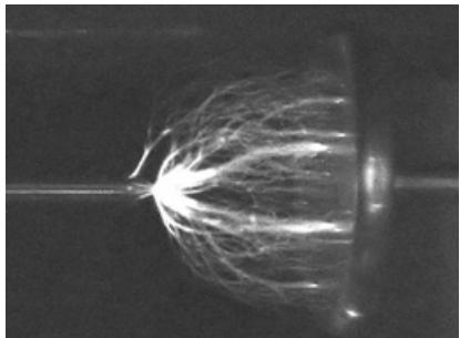
High voltage discharge between gas insulated (SF6 gas) conduits. With friendly permission of: Laboratory of High Voltage Engineering and Switchgear Technology, Technische Universität München, Munich, Germany [www.hsa.ei.tum.de](http://www.hsa.ei.tum.de)
