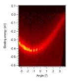
Cu (111) state dispersion image by a pco. pixelfly, courtesy of Specs GmbH - Surface Analysis and Computer Technology, Berlin, Germany
