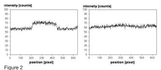
The graphs show the read out profiles of both aperture images in figure 1. The left graph clearly shows the step-like signal increases due to smear (smear approximately equal to 10-12 counts), while the dark value is similar for both images (58-62 counts).
