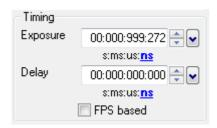
The exposure and delay time can be adjusted in steps of 1 µs.
