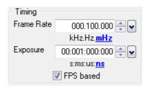
First the frame-rate is set. If the time required for readout of the image is longer than 1 / frame-rate, then the frame-rate will be reduced to 1 / treadout.
