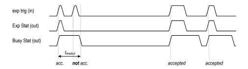
The detailed timing for external trigger includes system delay times, an adjustable additional delay time, and the jitter.
