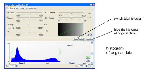
The user can influence how the 10 (12,14) bit intensity values (x-axis) of the original image are converted into 8 bit values (y-axis) in different ways.
