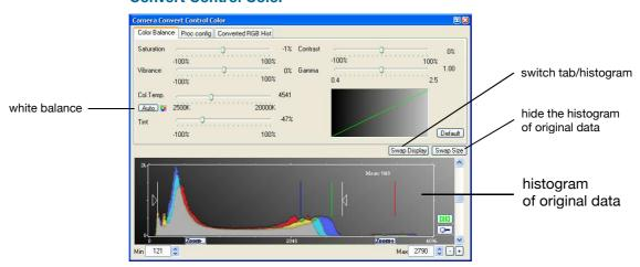
The user can influence how the 10 (12,14) bit intensity values (x-axis) of the original image are converted into 8 bit values (y-axis) in different ways.
