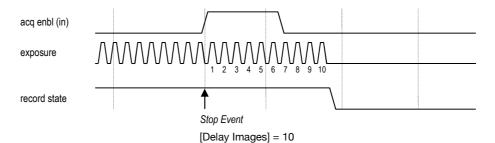
The relative position of the trigger within the recorded time window depends on the size of the RAM segment and the skip images parameters. The following figure shows one example, where the buffer size is 1000 images:
