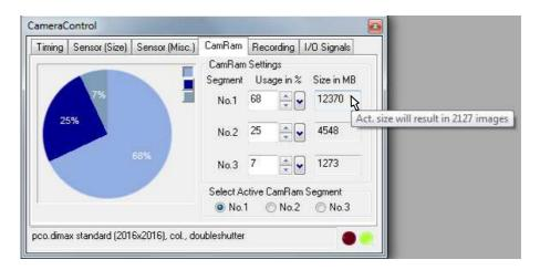
The CamRam tab is for controlling the camera built in memory (camRAM). You have the possibility to record into 3 different segments.
