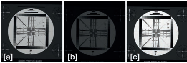
Figure 10 Images of the same test chart with same resolution, same object distance, same fill factor but different pixel size and different lens settings (all images have the same scaling for display): a) pixel size 14.8 μm x 14.8 μm, f = 100mm, f-number = 16 b) pixel size 7.4 μm x 7.4 μm, f = 50mm, f-number = 16 c) pixel size 7.4 μm x 7.4 μm, f = 50mm, f-number = 8
