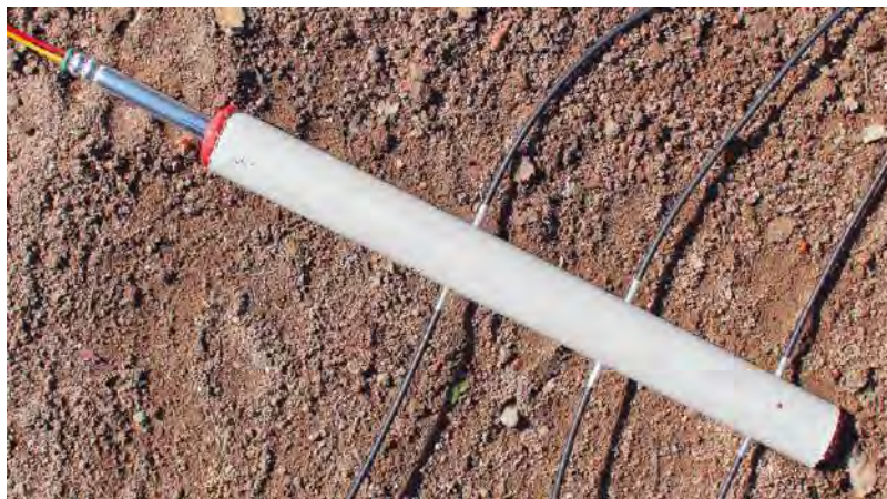
Measurement setup for a confined plastic explosive
