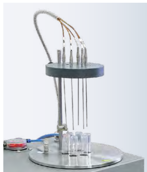
AET 402 – detail of the furnace
