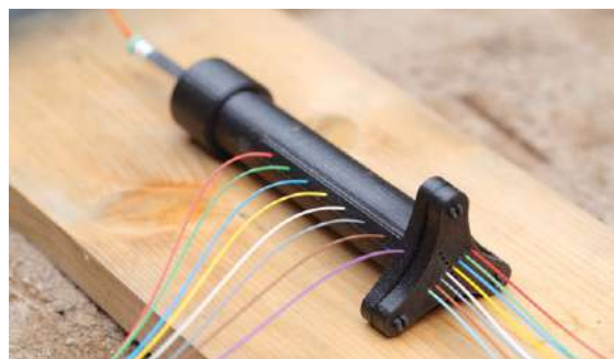
Simultaneous detonation velocity and shock curvature measurement
