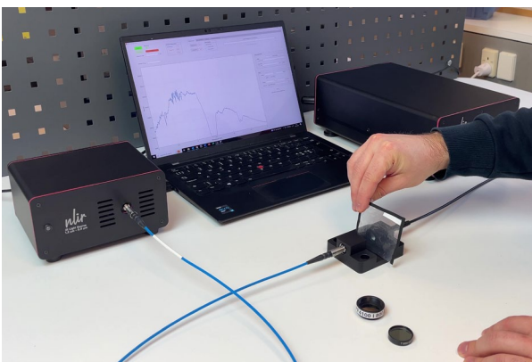
Foil characterization in Transmission Measurement System using NLIR's MIDWAVE Spectrometer, TRANSMISSION Interface and FIBER Light Source.
