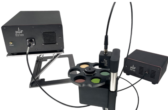
Optical coating characterization using NLIR's MIDWAVE Spectrometer COLLIMATOR Accessory and FIBER Light Source.
