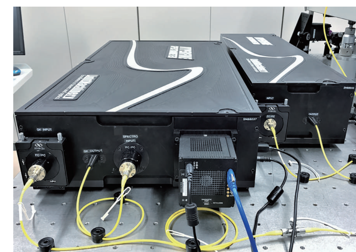
Brillouin HyperFine spectrometer with SMF input (LightMachinery)
