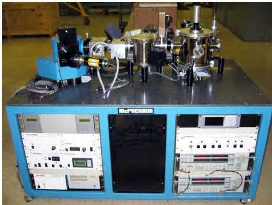
**VUVAS 2000 Vacuum Ultraviolet Analytical Spectrophotometer**
