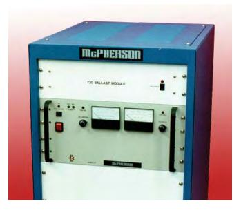
Voltage and current regulation are exceptional with ripple better than 0.1%. The unit is protected by automatic regulating circuitry along with fuses and surge resistor components that are built into the unit.
