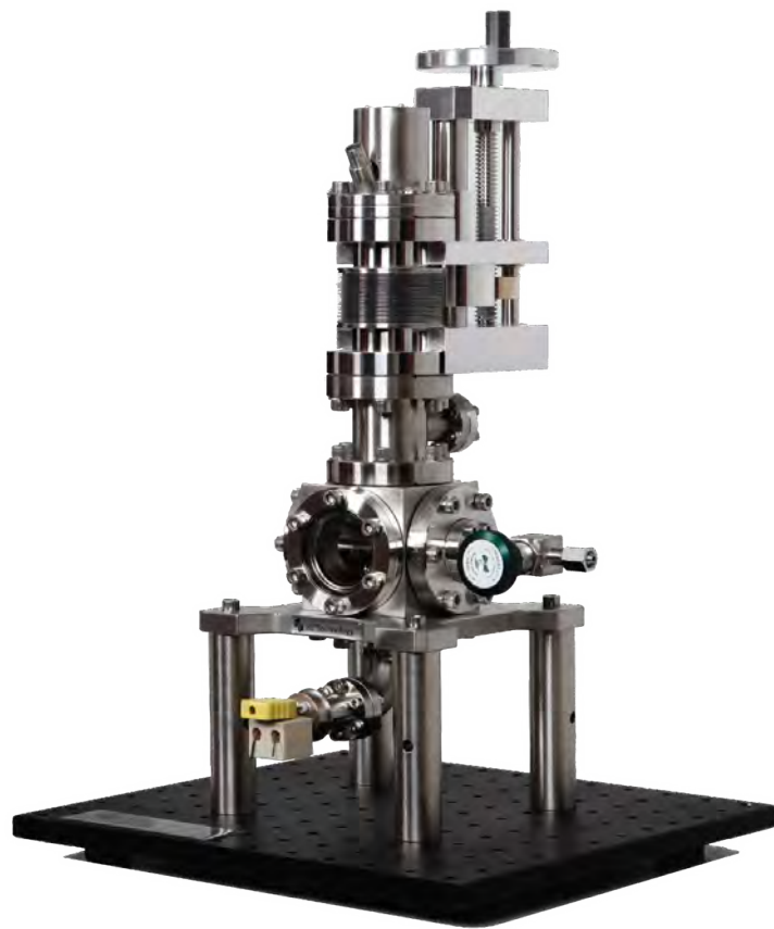
UHVKP corner cube system, mounted on breadboard. Cell with heater stage, gas inlet and Kelvin probe mounted vertically.
