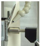
friction movement. Located between specimen and test piston a specific standardized fabric guarantees constant standardized friction.
