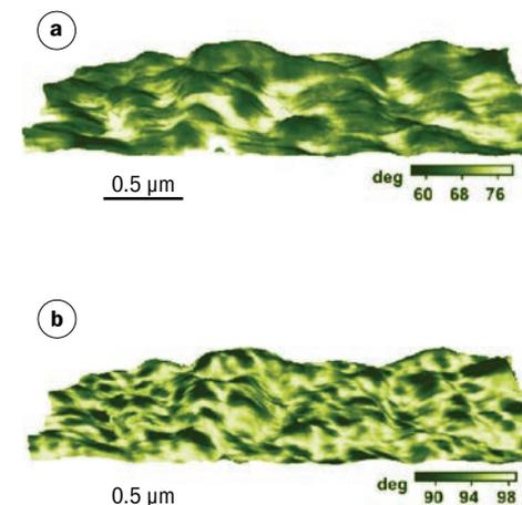
In figures (a) and (b) the phase data from repulsive and attractive regimes, respectively, have been overlaid on the corresponding topography image. Features of the phase contrast in the repulsive regime correspond to some features in the topography, while the phase contrast in the attractive regime is independent of the topography. Images were taken with the NSC15/AIBS (now upgraded to HQ:NSC15/Al BS). (O'Dea, J.R. and Burrato, S.K.; J. Phys. Chem. B 2011, 115, 1014-1020.)
