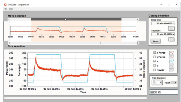
Fig.2 Stress-relaxation force signatures (red) for 1 trap during two indentation steps (trap movement in blue). Visualized with SyncData tool.
