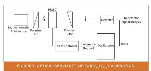
In general, this experimental setup should resemble as closely as possible the optical bench setup for the experiment in question. Some additional precautions need to be mentioned. First, if the light source is a laser, the effects of modulated interference must be minimized or eliminated.5 Second, the polarizers should be of high quality (such as Glan-Thompson calcite polarizers) with very good extinction characteristics.
