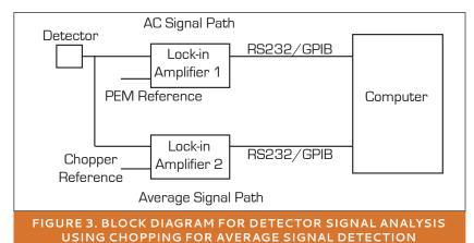
Lock-in amplifier I must have frequency response capable of accepting the polarization modulated signal at the modulator frequency f and twice this value, 2f. A lower frequency model lock-in (probably less expensive) may be used for lock-in 2.
