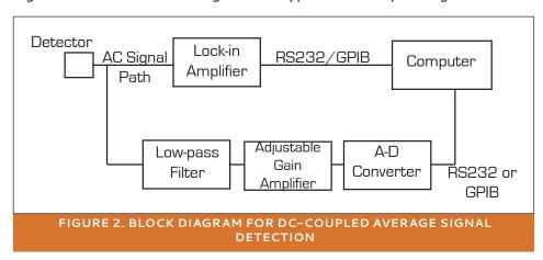
Another approach to average signal detection would be to use a digital voltmeter (DVM) connected to the output of the detector in parallel with the lock-in amplifier. Many such instruments are equipped with RS-232 or GPIB interfaces. In decidina
