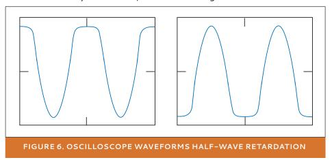
The characteristic flat top (or flat bottom) of this waveform can be used to establish that the PEM has been accurately adjusted to half-wave retardation. (See the Calibration Application Note.) <sup>7</sup> For  $A_0 = \pi$ ,  $J_0(\pi) = -0.30424$  and  $J_2(\pi) = 0.48543$ , giving
