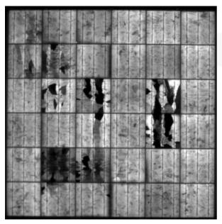
Electroluminescence image acquired using a C-RED 3 camera.
