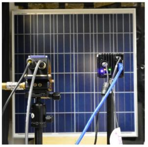
Laboratory set-up using a C-RED 3 camera (right) and a laser module (left) for photoluminescence imaging of a PV panel
