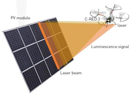
Schematic of the full LIPI system in operation.
