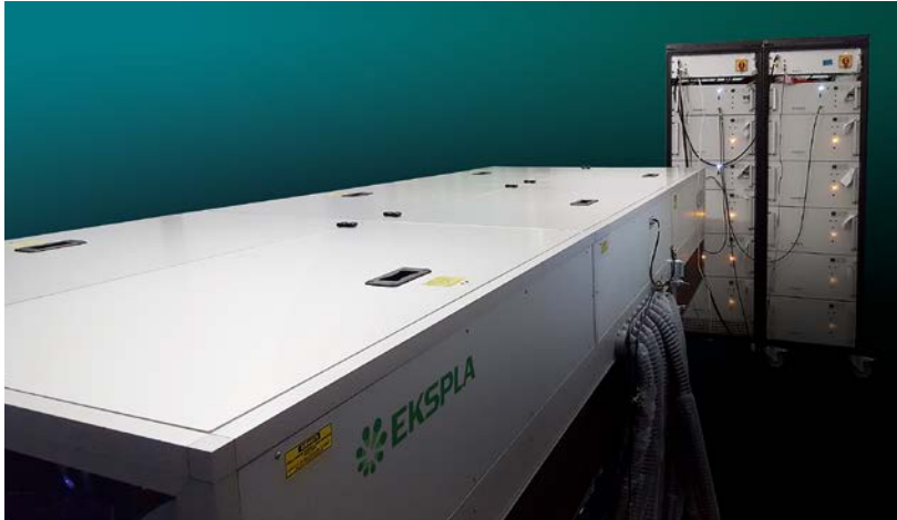
Typical external view of ANL80KSS-AWG laser system
