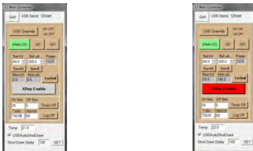
Figure 16: MagPro control software showing it after initialisation (left) and when the source has been started (right)
