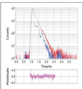
Erythrosin B in water, excitation by supercontinuum laser at 520nm, detection by MCP-PMT at 560nm. The calculated lifetime is (88±2) ps, with a goodness of fit quality parameter ( $\square^2$ ) of 1.180.
