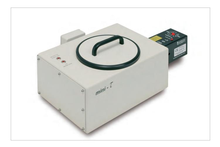
The Mini-tau is an ultra-compact, low cost, filter-based dedicated fluorescence lifetime spectrometer. Using the Time-Correlated Single Photon Counting (TCSPC) technique, the Mini-tau can measure fluorescence lifetimes ranging from 25 ps to 10  $\mu s$ . It can also be equipped with Multi-Channel Scaling (MCS) electronics for long-range photoluminescence from 10 ns to 10 s.
