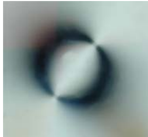
FIGURE 6 Pattern which is observed when looking off-axis through two \theta -cells in between polarizers.
