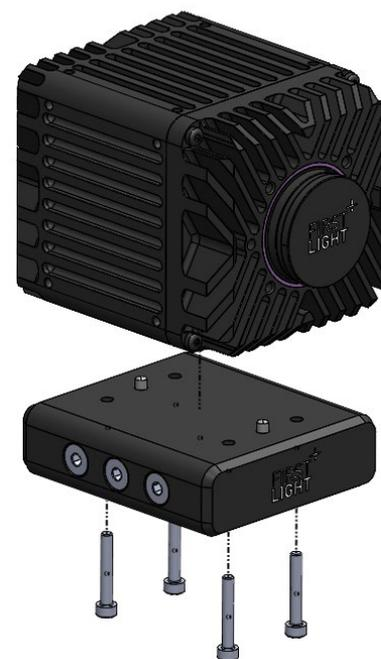
*Schematic of hydraulic cooling plate installation*
