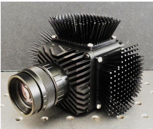
*Passive heat sinks set-up*
