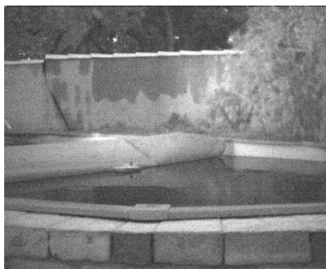
Night vision in the SWIR range. Imaging of a boat in a swimming pool, by a moonless night. Camera used: C-RED 2 with SWIR lens 16 mm, cooled down to -15°C, High gain.
