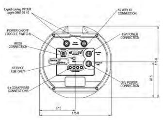
Note: air vents are not present in the housing of the Liquid Cooled Only model (not shown). This option can be selected for minimal thermal bloom.
