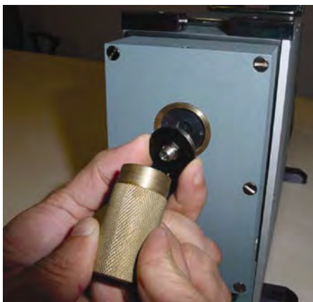
Figure 31: Fitting SMA connector over Slit Disc
