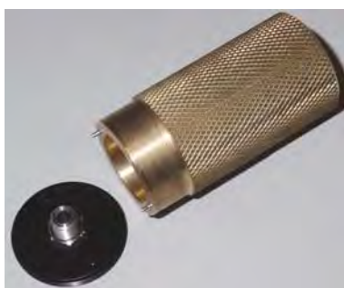
Figure 27: SMA connector & brass insertion tool
