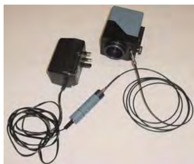
Figure 41: Aiming laser fitted to Collector/Collimator
