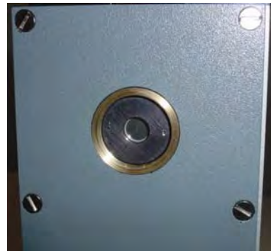
Figure 30: Shutter housing fitted with Slit Disc only
