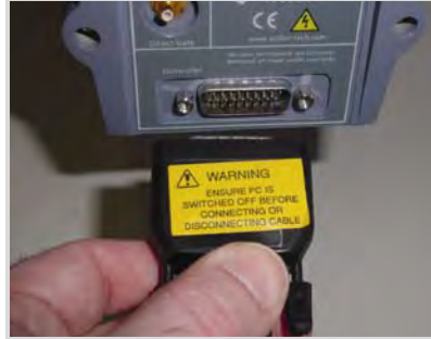
Figure 5: Connecting Interface cable to camera ( please note warning on label )
