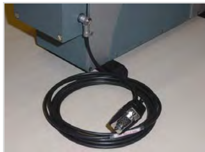
Figure 6: Shutter/Temperature cable connected to Mechelle
