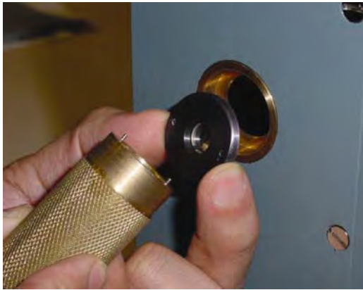
Figure 29: Inserting Slit Disc
