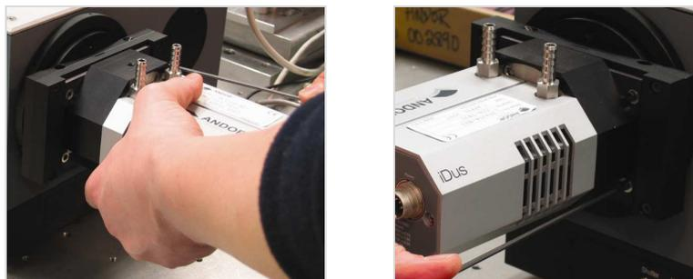
3. Loosen the rotation locking screws, e.g.:
