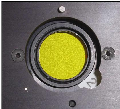
**NOTE:** The filter position accessible via the access hole has an ID number 2 less than the filter position in the optical path, and the number displayed in the software (e.g. filter position 2) will be accessible via the access hole when filter position 4 has been selected in the software (i.e. 2 → 4).
