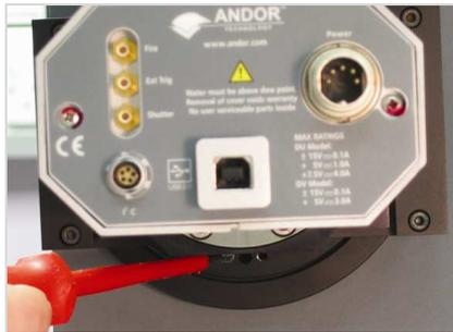
6. Finally, check that the focusing ring is free to rotate, e.g.:
