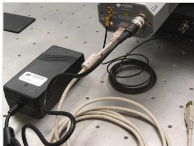
Connections showing PS-24 Power Supply
