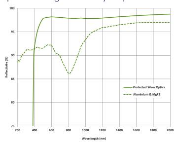
Standard systems use Al +  ${\rm MgF_2}$  coated optics. Protected silver optics are also available on request for maximum efficiency in the NIR region - recommended for working with Andor iDus InGaAs detectors or IR single-point detectors, such as MCT, PbS and InSb.
