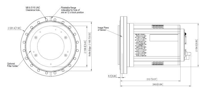
Dimensions in mm [inches] Weight (approx): 9.5 kg [20lbs 150z], (9.7 kg [21lbs 60z] with filter holder)
