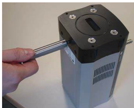
Figure 2: Fitting mounting posts (NOTE: Shown on an Andor Newton camera)
