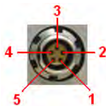
Figure 11: I²C connection (facing in) with pinouts
