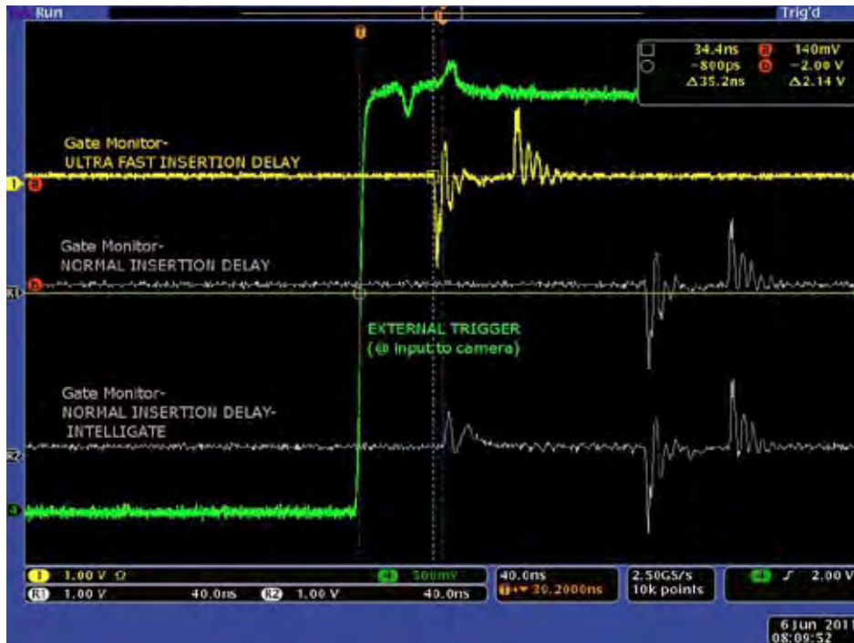
External Trigger to intensifier opening using DDG
