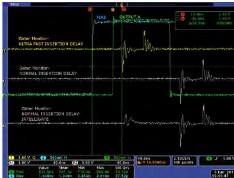
Fire pulse to intensifier opening using DDG
