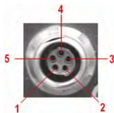
Figure 5: I 2 C connection (facing in) with pin-outs
