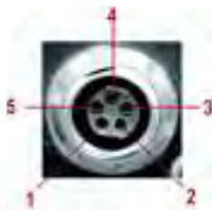
Figure 5: I 2 C connection (facing in) with pinouts
