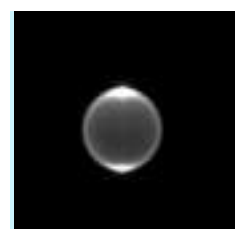
Beam perfectly focused on BFP. Perfect TIRF
