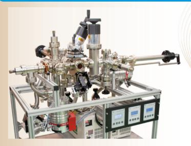
HEMTO-TDS is a thermal desorption spectroscopy (TDS) system designed to detect trace amounts of hydrogen from small-volume samples such as thin films. The highly hydrogen-sensitive detection is achieved by combining the efficient sample heating by infrared laser with the extremely low hydrogen background level maintained by a BeCu chamber. Equipped with a quadrupole mass spectrometer (QMS), the HEMTO-TDS is the ideal instrument for analyzing hydrogen with other desorbed gases.
