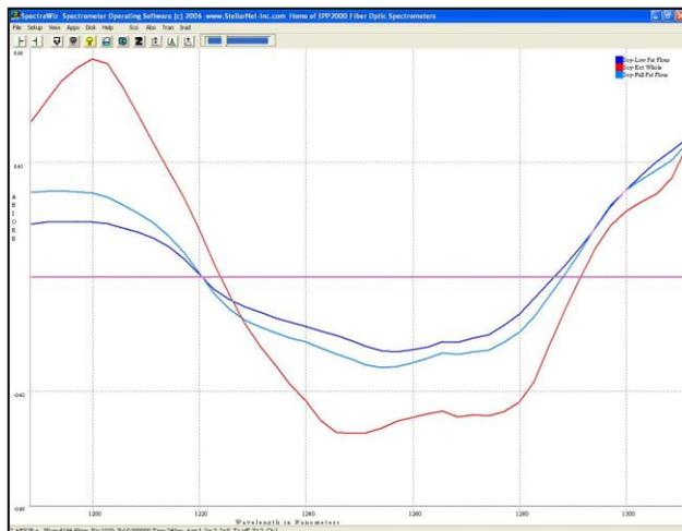
**RED-Wave-NIRx-SR-InGaAs-512 spectrum showing 2<sup>nd</sup> Derivative spectral reflectance data of various soybeans (whole, low-fat, and full-fat). The RFX-1 integrated sampling accessory/light source was used for simple reflectance measurements with no sample prep required.**
