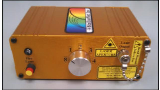
RamuLaser accessory attaches to Raman probe
