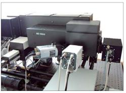
New type of 520 mm focal length spectrometer with 3 exit ports
