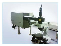
chamber or cryostat is also available. Sample imaging can be realized by moving the laser beam with a Galvano mirror scanner.
