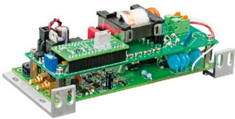
PCD-UHV driver mounted with HV power supply HV05Wm
