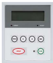
Fig. 2. Front panel controls of PS5050 flashlamp driver
