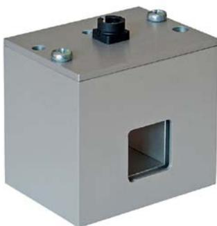
CH4 oven has identical mechanical design as CH3. The pre-set temperature can be adjusted in  $\pm 5$  °C range by the help of potentiometer. The current temperature is not indicated. In addition, CH4 has “temperature ready” output signal, changing state when pre-set temperature is reached. CH4-50 model can fit crystals with up to 50 mm length.
