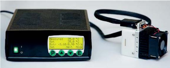
With combination of temperature controller, CO10 series ovens are designed specifically for tuning and conditioning the periodically poled bulk devices (PPSLT, PPLN & PP-MgO:LN) and other nonlinear crystals. The oven is designed to hold the crystal with dimensions of 30×16×1 mm. Custom made oven is also available. The crystal heater provides temperature stabilization for crystals with an accuracy of 0.1°C. The crystal temperature can be changed from 50°C to 200 °C.
