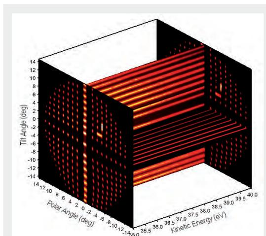
Demonstration of the PHOIBOS 150 SAL 2D angular resolution in dependence of the electron kinetic energy.
