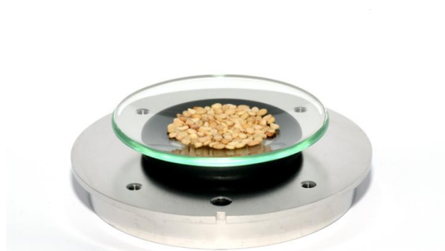
Fig. 1 Untreated, organic sesame seeds in a watch glass on an EnviroESCA sample plate
