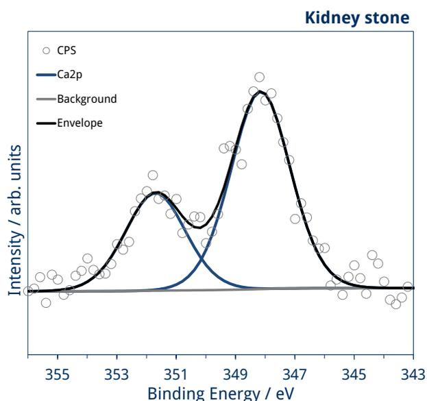
Fig. 6 Ca 2p core-level spectrum of a urinary (kidney) stone
