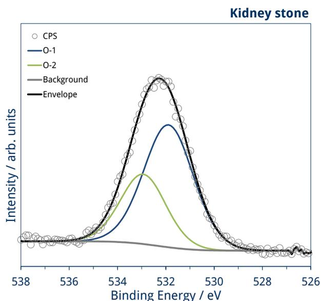
Fig. 5 O 1s core-level spectrum of a urinary (kidney) stone
