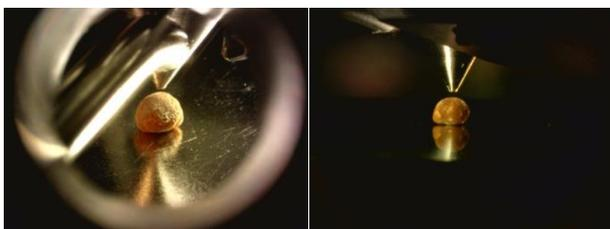
Fig. 1 Urinary stone underneath the analyzer nozzle at a working distance of 0.3mm
