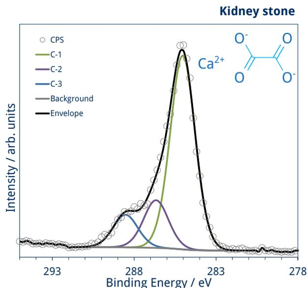
Fig. 7 C 1s core-level spectrum of a urinary (kidney) stone with the chemical structure of calcium oxalate (inset)
