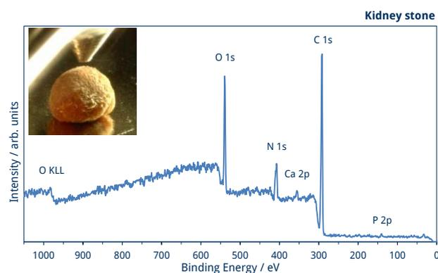
Fig. 4 Survey spectrum of a kidney stone
