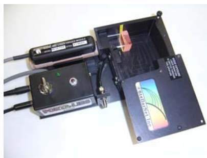
Figure 2. The LIBS system. The entire platform, including the laser, sample compartment, and trigger module measures 5 cm x 21 cm x 10 cm. Not shown is the battery pack or the laptop computer.
