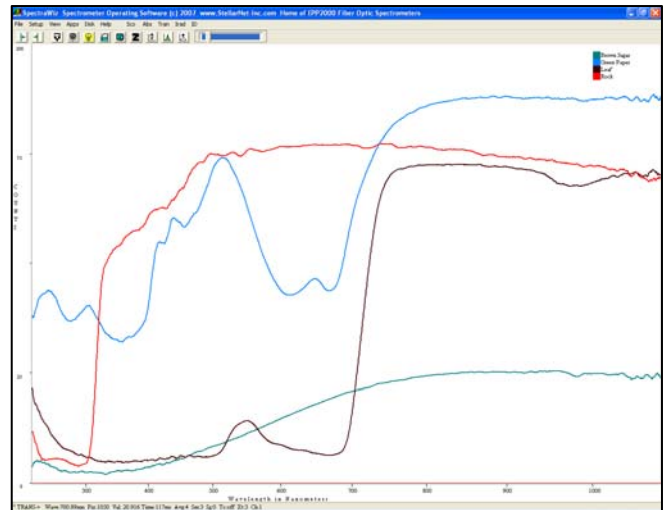
Paper, leaf, powder, and rock spectra obtained with the SL4-DT and concave grating spectrometer
