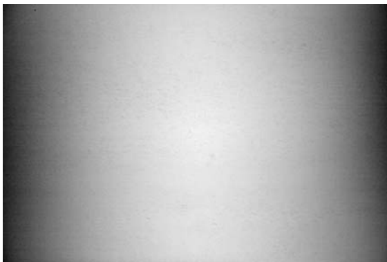
Figure 4: The image is identical to the right image in figure 3 only that the scaling is different to better illustrate the shading effect. The scaling is 9280-15519 counts correspond to 0-255 gray levels, which is a minimum/maximum scaling.
