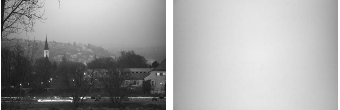
Figure 3: Both images have been recorded with a KAI-11000 image sensor and a Nikkor 1.8/105mm lens at an f-stop of f/8 . The left image shows a normal scene and the right image shows a homogeneous illuminated area. Both images are scaled to full scale, such that 0-16384 counts correspond to 0-255 gray levels.
