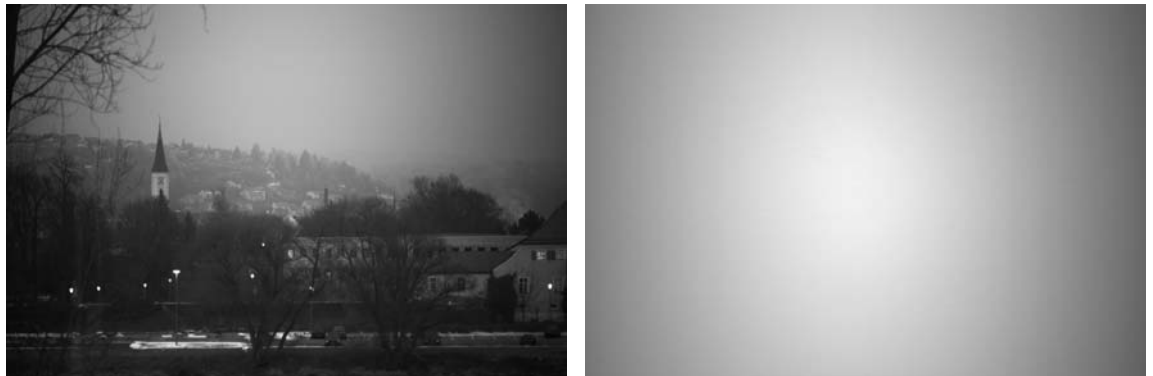
Figure 1: Both images have been recorded with a KAI-11000 image sensor and a Nikkor 1.8/105mm lens at an f-stop of f/1.8 (open aperture). The left image shows a normal scene and the right image shows a homogeneous illuminated area. Both images are scaled to full scale, such that 0-16384 counts correspond to 0-255 gray levels.
