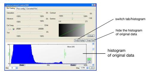
The user can influence how the 14 bit intensity values (x-axis) of the original image are converted into 8 bit values (y-axis) in different ways.
