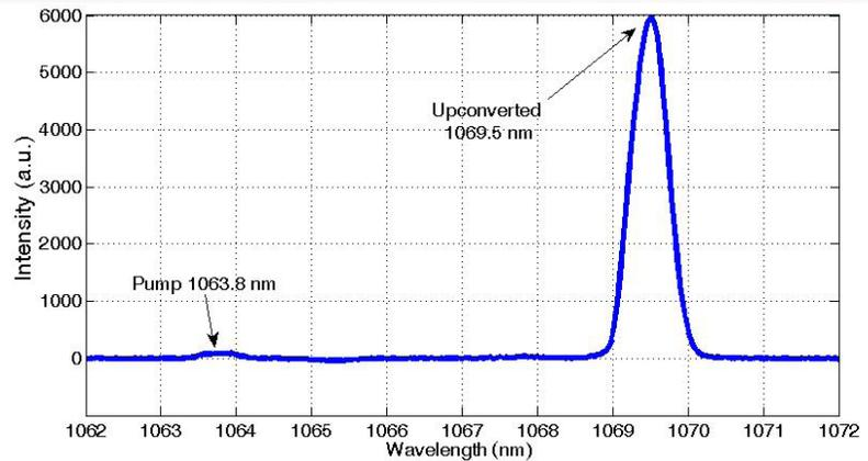
As with any nonlinear interaction, the efficiency of the up-conversion process increases with peak power. For this reason shorter pulses offer the advantage of higher signal powers. By keeping the bandwidth narrow, the spectrum of the up-converted signal can be well separated from the strong IR light (figure 2), which enables spectral filtering of the background.
