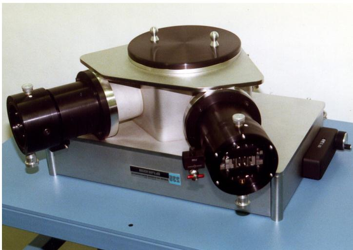
Stainless steel construction makes this proven design suitable for use with high vacuum, contaminant free experiments or microchannel plate intensifiers. Wavelengths from 30-nm to 1.2-um can be covered within the scanning range and with appropriate gratings. The 235 is for scanning and microchannel plate intensifier or CCD spectroscopy.
